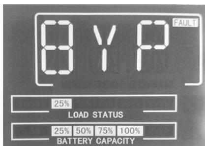
**Figura 2-19** Falla de bypass
